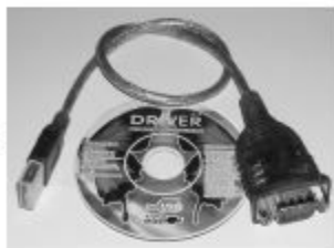
Fig R2 A Sabrent® USB/RS232 cable adapter using a Prolific chipset.
